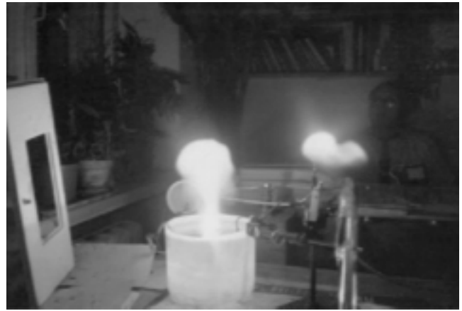
Fig. 2. Generation of two LOs in the same discharge. The second LO (on the right) is located near the copper rod.
